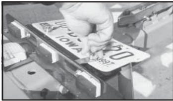
Step 3. Loosen wing nut on back of license plate holder, turn the clip on the front to a horizontal position and put license in the "down" position. Turn the clip back so it rests against the back of the light bar to hold the license down and tighten wing nut.
